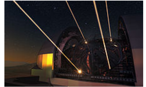
Artist's impression of the European Extremely Large Telescope deploying lasers for adaptive optics [11]
