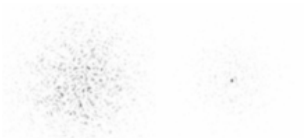
Negative images of a star through a telescope. The left-hand panel shows the slow-motion movie of a star when the adaptive optics system is switched off. The right-hand panel shows the slow motion movie of the same star when the AO system is switched on.
