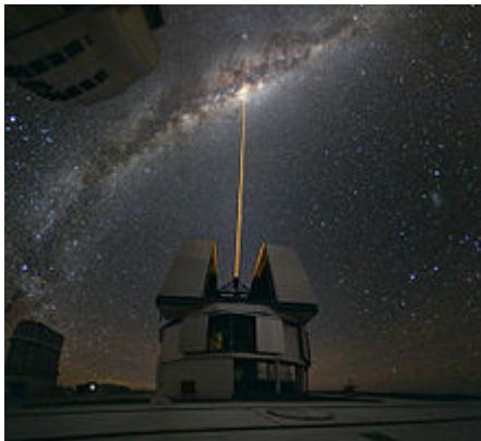
A laser beam directed toward the centre of the Milky Way. This laser beam can then be used as a guide star for the AO.
