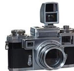
Contax III rangefinder camera with macro photography setting. Because the viewfinder is on top of the lens and of the close proximity of the subject, goggles are fitted in front of the rangefinder and a dedicated viewfinder installed to compensate for parallax.
