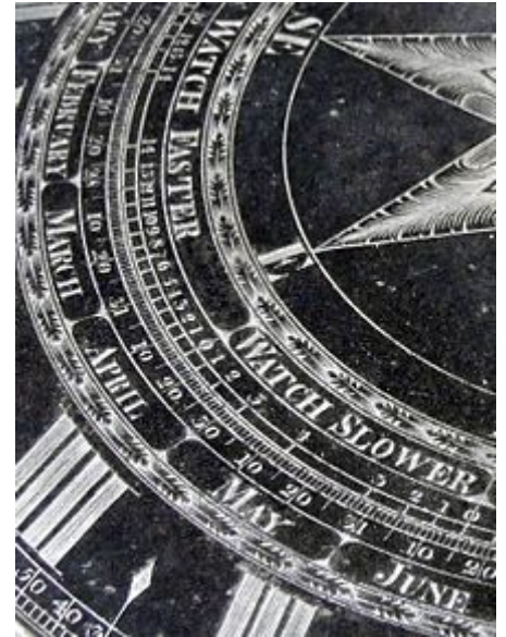
A sundial made in 1812, by Whitehurst & Son with a circular scale showing the equation of time correction. This is now on display in the Derby Museum.
